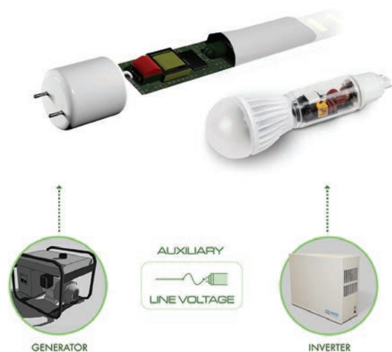
Fig.2 - LED tube lamps with internal drivers do not require a fluorescent ballast. When no external ballast is available to wire the emergency ballast to, an auxiliary supply such as a generator or inverter must be used to provide emergency line power.
